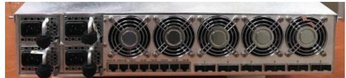
**The SR-60 comes integrated with a KVM-over-IP system, 12 10 Gb SFP+ ports and 6 1Gb auxiliary NICs.**
